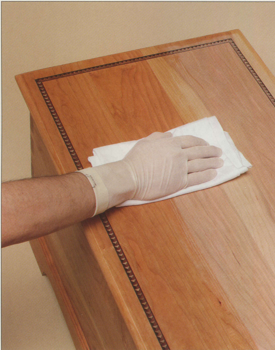
Easy to apply, a coat of polymerized tung oil is wiped onto the surface of this cherry toy chest, protecting the wood and giving it a warm luster.
