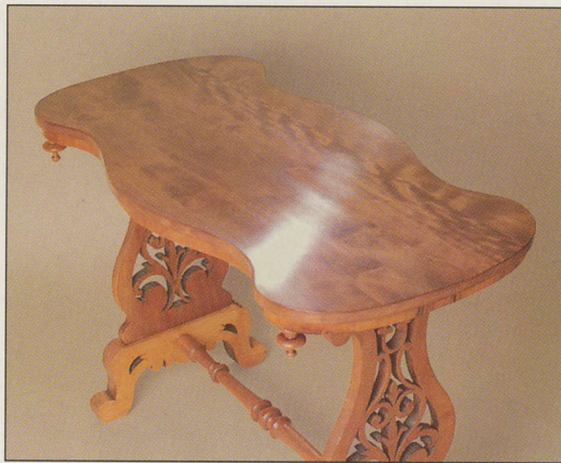
The varnish topcoat on this 19th-Century farmhouse-style table was rubbed out with extra fine steel wool and buffed with paste wax.
