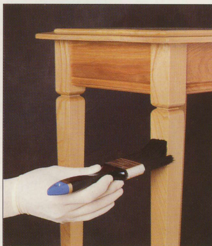
A varnish topcoat brings out the luster of an oak table. Finishing a piece by hand demands care. Loading the brush with too much finish, particularly when coating vertical surfaces, can result in drips and runs.
