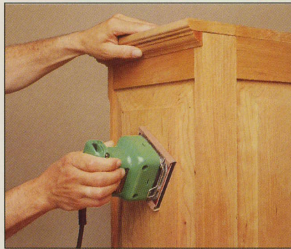
Combining the convenience of a power tool with the fine touch of hand sanding, a palm sander readies a cabinet for a finish.
