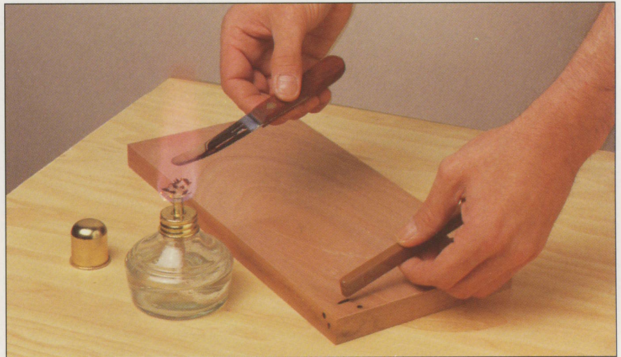
A traditional shellac stick remains one of the best methods of repairing minor damage in wood. Heated by the flame from an alcohol lamp, a burn-in knife melts a small bit of the shellac stick, which fills the hole level with the surface.
